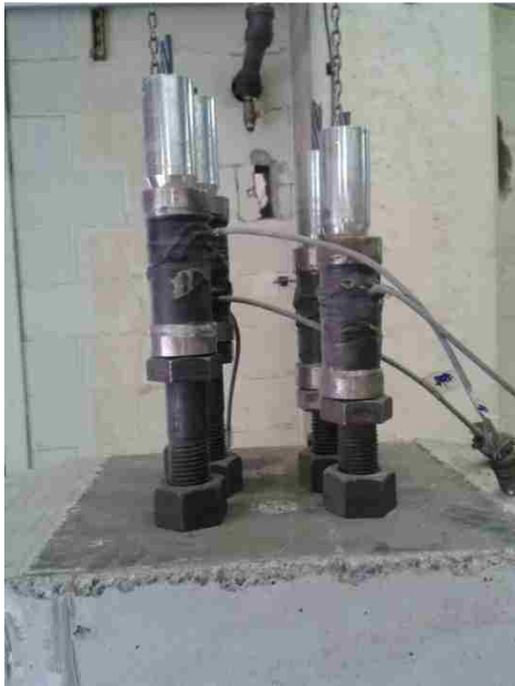
Figure 2.5 Photograph (Left) and schematic (Right) views of the system to detect and prevent the strands from slipping.
