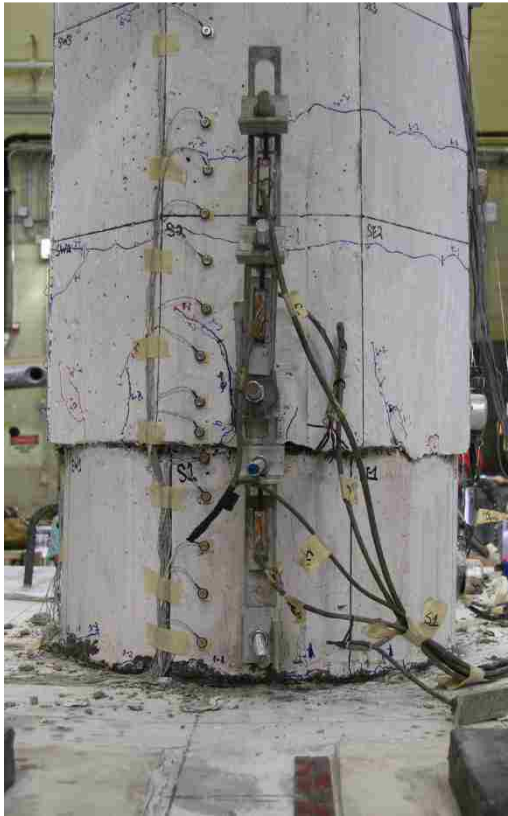
Figure 4.4 South view of PreT-SF-ROCK after cycle 9-1 (6% max drift) showing hairline cracking in the column.
