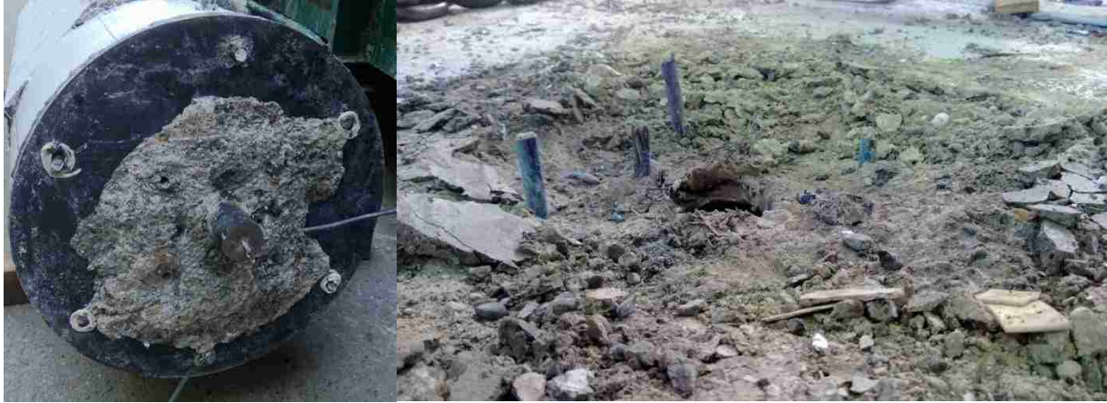
Figure 4.8 Jagged portion of HyFRC that seeped through steel-wire mesh (Left). Column-footing interface after top portion of column was removed (Right).
