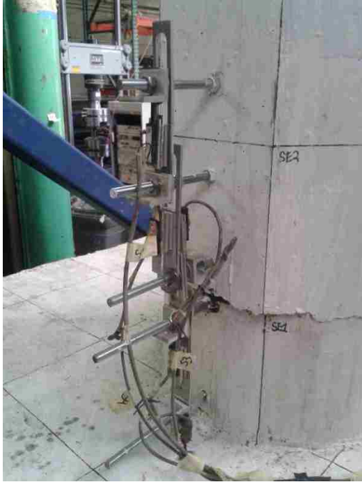
Figure 3.6 Photograph (Left) and schematic (Right) views of the curvature rod system used on the north face.
