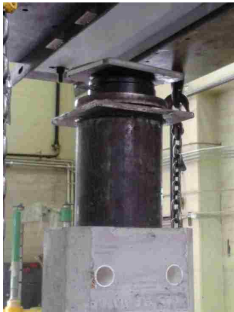
Figure 3.2 Actual (Left) and Schematic (Right) views for the system that transfers load from the Baldwin to the specimen while safely covering prestressing load cells and chucks.
