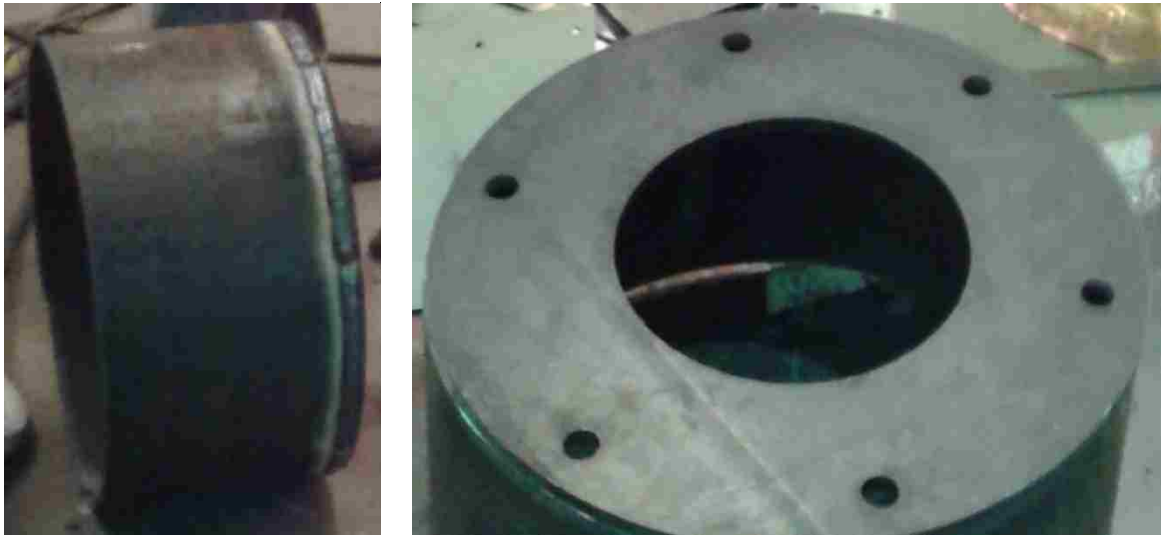
Figure 2.6 Steel shoe. On left is an elevation view of the shoe while on right is a bottom view of the shoe.
